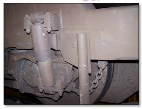
2. Check the underside of truck frame around the 4 inch hole for any irregularities. If needed, grind off any areas so that spacer fits flat on surface inside the frame.
