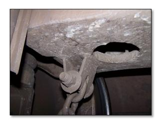
3. Insert 6.5" bolt in the mounting plate support and insert it through the 4 inch hole. Ensure that
