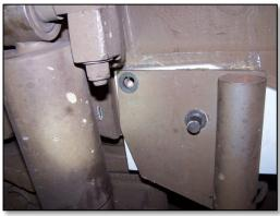
6. Attach the mount bracket to the adjustable tube and tighten using provided hardware. Install adjustable tube into the mounting bracket.
