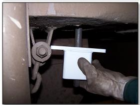
Reinstall sand pipe mounting plate and remove upper dowel. Install the 2.25 inch bolt and flat washer into the upper hole and tighten. Remove lower dowel, insert remaining 2.25 inch bolt and flat washer and tighten.
