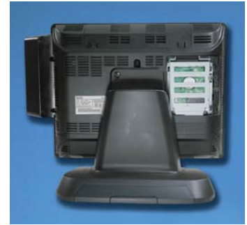
Tool-Free Access to Compact Flash or Hard Disk Drive Optimizes Serviceability
