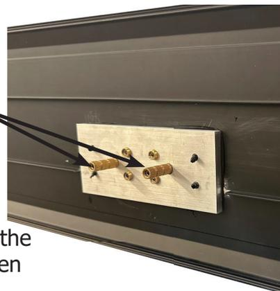
Apply glue to the bottom of the metal plate. Add glue in the holes in the floor. Make sure the holes don't overflow when you place the floor plate.
